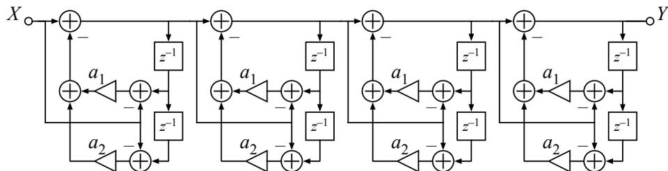
Figure 9.16: A 4th-order APGF constructed as shown, using the modified direct-form two-pole stage of Figure 8.18, always has unity gain at DC, no matter how the poles are moved via the  $a_1$  and  $a_2$  coefficients.
