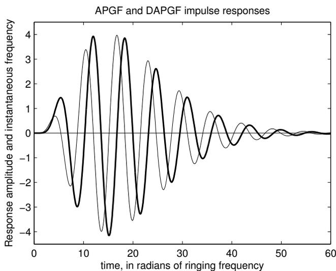
Figure 9.7: Impulse responses of the 4th-order all-pole gammatone filter (APGF, heavy curve) and its derivative, the DAPGF (light curve), with pole damping  $\zeta = 0.2$  ( $Q = 2.5$ ,  $Q_{3dB} \approx 5$ ).
