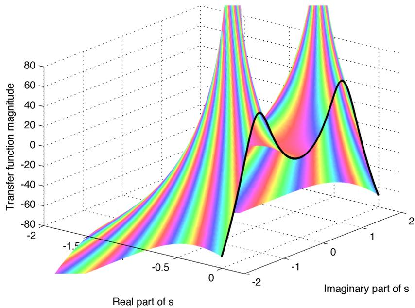
Figure 9.13: The complex transfer function for the Kim et al. filter. The cut line on the imaginary  $s$  axis shows the log-magnitude transfer function, with zero frequency in the center. The phase (hue) goes through 10 cycles around each cluster of 10 poles.
