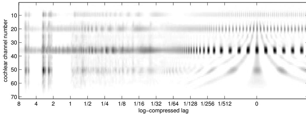
Figure 21.22: An SAI frame of a telephone ringing (file *BelgiqueBellPhone.mp3* from [freesound.org](http://freesound.org)), with longer lags logarithmically compressed. The telephone sound exhibits structure on many time scales, out to its 3 s period and 6 s double period, and has somewhat different structure in different frequency regions.
