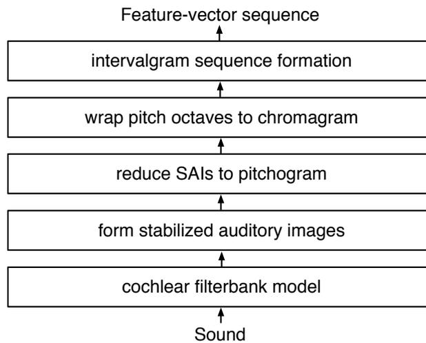
Figure 25.1: This multistage feature extraction pipeline for melody matching, described in detail in Chapter 27, maps into the first three levels of our *four-layer model* of Figure 1.5. Some of the stages here could alternatively be pushed into the uppermost layer, the machine learning system, with the possibility that they would be end-to-end optimized for the application.
