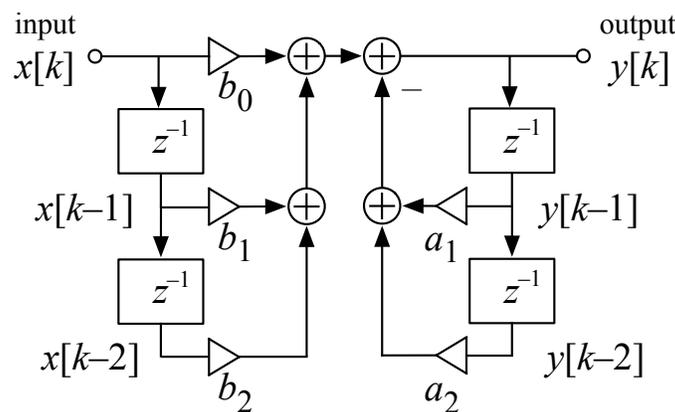
Figure 7.5: The signal-flow diagram of a second-order digital filter with three forward coefficients and two feedback coefficients. The filter’s difference equation  $y[k] = b_0x[k] + b_1x[k - 1] + b_2x[k - 2] - a_1y[k - 1] - a_2y[k - 2]$ , which is apparent from the diagram, is also the program step that computes an output sample.
