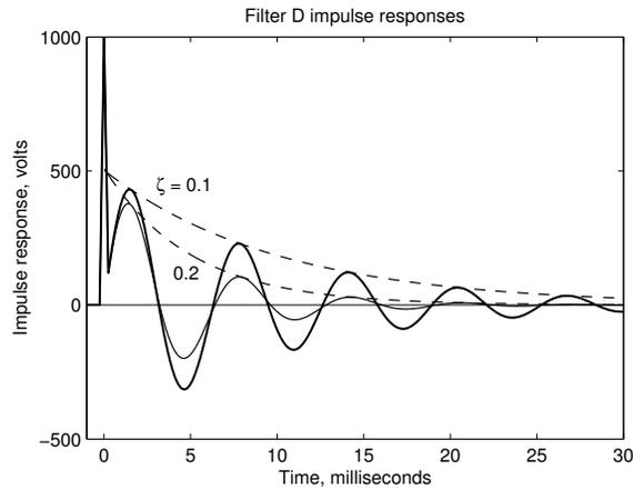
Figure 8.15: The impulse responses of the asymmetric resonator, filter D, contain an impulse of weight  $a$  (illustrated here with  $a = 0.5$ ) at  $t = 0$ , representing the straight-through path. Since an impulse is infinitely tall and narrow, it is approximated in this plot by a triangle, of base width 0.001 s and height 1000, with the correct total area 0.5. Impulse responses for two dampings are shown, with the envelopes (dashed) of the exponentially decaying portions.
