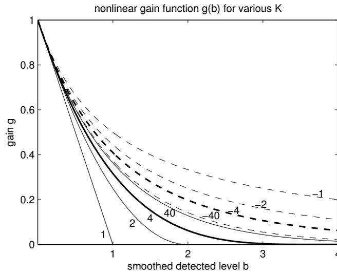
Figure 11.3: The family of nonlinear gain functions  $g(b)$  used in the AGC analysis, for various values of the  $K$  parameter. All functions are near  $1 - b$  at low levels, but their high-level behavior depends on the parameter. Negative  $K$  values are represented with dashed curves;  $|K| = 4$  curves are bold, representing typical system choices. For high  $|K|$ , the functions approach  $g(b) = \exp(-b)$ .
