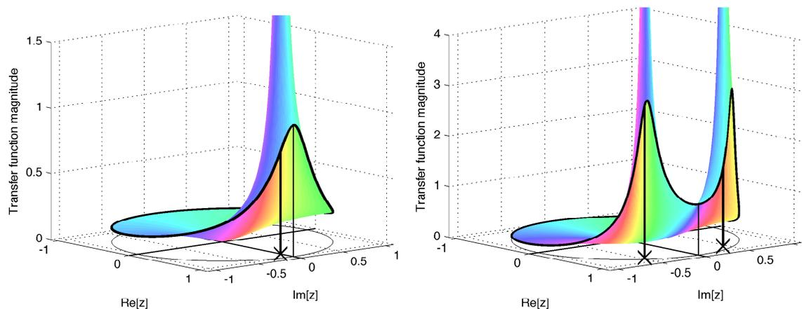
Figure 7.2: Complex transfer functions of one-pole (smoothing) and two-pole (resonator) filters, evaluated inside the unit circle of the  $z$  plane. The frequency response is the transfer function evaluated on the unit circle, shown by the dark curves at the circular cut. As in Figure 6.4, phase is mapped to hue (see the color plates); there is one cycle of hue variation around each pole.
