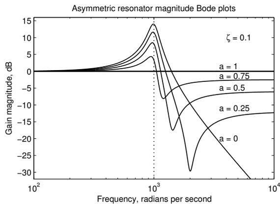
Figure 8.16: Bode plot for the asymmetric resonator with variable mixing ratio. The weight of the “straight through” signal is  $a$ , and of the two-pole resonator is  $1 - a$ . This parameter interpolates between a flat response at  $a = 1$  and the response of the simple resonator at  $a = 0$ , resulting in a cancellation dip above the peak.
