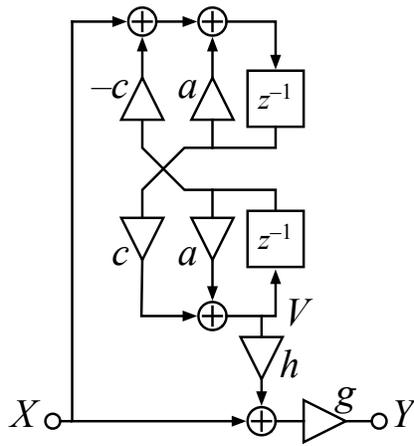
Figure 8.21: A pair of zeros is added to the coupled form by mixing the input with a minimum-phase all-pole filtered version, as in filter D.
