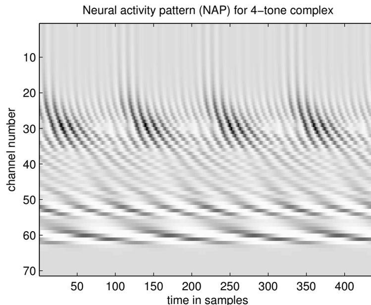
Figure 18.8: The neural activity pattern (NAP), the response of a bank of DIHCs in the context of the CAR-FAC, with the 4-tone stimulus of Section ??, at 60 dB SPL. The NAP represents, at least conceptually, the instantaneous firing rates of the groups of primary auditory neurons attached to each IHC.
