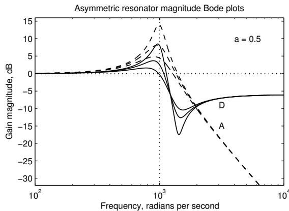
Figure 8.14: Bode plot for the asymmetric resonator (filter D, solid), compared to the all-pole resonator (filter A, dashed), for damping factors 0.1, 0.2, and 0.4, with mixing weight  $a = 0.5$ . The zeros cause an *anti-resonance* or *notch* about a half octave above the resonance. The high-frequency asymptote is flat, which means the impulse response will contain an impulse.
