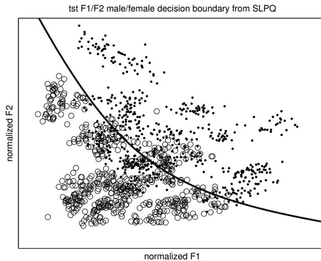
Figure 24.5: A feature-space map showing the decision boundary of a single-layer perceptron classifying talker gender from  $F_1$ – $F_2$  data, when the input feature vector is augmented with three quadratic dimensions (two squares and a cross term). The nonlinearities at the input help, but only a little; test-set errors are reduced to 247, from the 267 of Figure 24.2.
