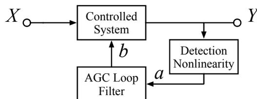
Figure 11.1: A system with automatic gain control (AGC). The loop filter output,  $b$ , can control any parameter of the controlled system that affects its gain. The loop filter, in combination with the properties of the controlled system and the detector, determines the dynamics of the response to a change in input level.
