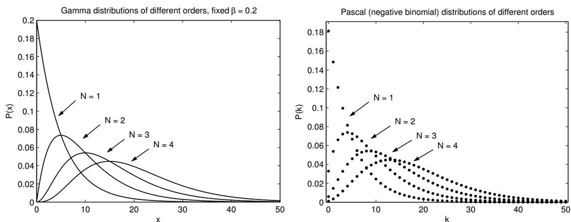
Figure 9.2: On the left are the impulse responses of cascades of  $N$  identical continuous-time one-pole smoothing filters, which are also gamma or Erlang distributions, for several values of  $N$ . On the right are impulse responses of cascades of  $N$  identical discrete-time one-pole smoothing filters with time constants of about 5 samples, which are also Pascal or negative binomial distributions of nonnegative integers.
