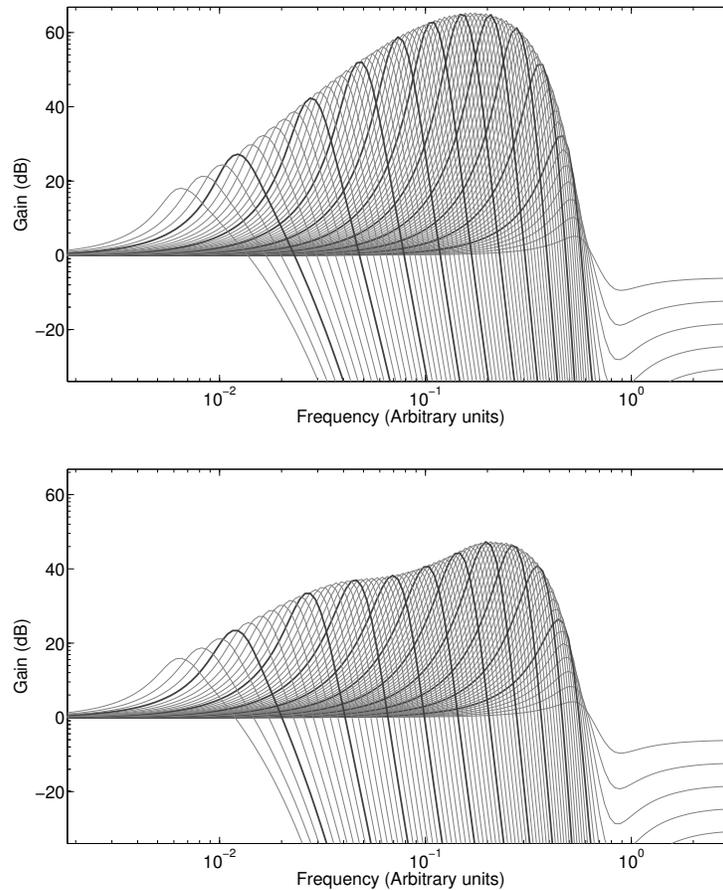
Figure 14.11: Adaptation of the overall filterbank response at each output tap, for the PZFC model of Lyon et al. (2010). The upper plot shows the initial response of the filterbank before adaptation. The lower plot shows the response after adaptation to a human /a/ vowel of 0.6 sec duration. The plots show that the adaptation affects the peak gains (the upper envelope of the filter curves shown), while the tails, behaving linearly, remain fixed.
