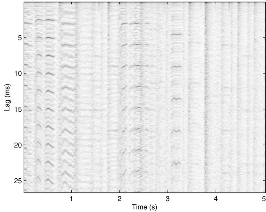
Figure 27.2: A pitchogram created by stacking a number of SAI temporal profiles in time. The lag dimension of the auditory image is now on the vertical axis. Dark ridges are associated with strong repetition rates in the signal.
