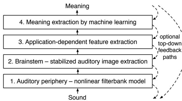
Figure 1.5: The *four-layer model* of machine hearing systems developed in this book—from sound to meaning, and sometimes back the other way. The big feedback loop from meaning to sound is for a system that can make sound and hear itself, for example, a speech conversation system.
