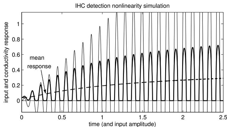
Figure 18.3: A simulation of the output of the rational-function detection nonlinearity of Figure 18.2 (heavy solid curve), when it is driven by an increasing-amplitude sinusoidal input (thin solid curve); this output function of time is the conductance  $g(t)$  used in the digital IHC model of Section ???. The mean response (dashed curve) is also shown; for the purpose of this illustration, the mean is taken over many phases of the input sinusoid.
