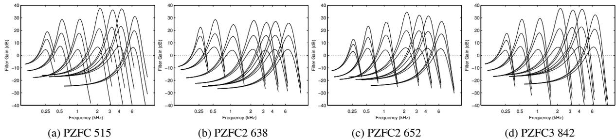
Figure 13.10: Auditory filter gain plots for several PZFC model types, including the PZFC2 and PZFC3 versions of the PZFC+ with different constraints on the zero positions relative to the pole positions.
