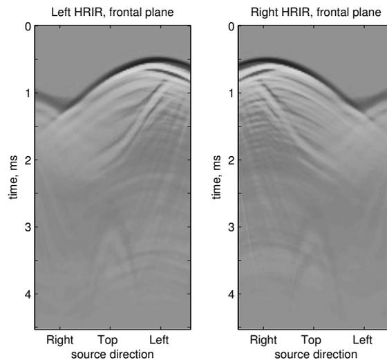
Figure 22.6: Head-related impulse responses of a dummy head, for sounds from various directions in the frontal plane. The  $x$  axis represents the angle of the sound source, from low on one side, over the top of the head, to low on the other side. The steeper patterns near the center, in the 1–2 ms range, represent shoulder-bounce arrivals, mostly at the ipsilateral ear, up to about 1 ms delayed from the main arrival (Brown and Duda, 1998).
