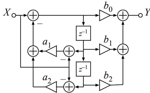
Figure 8.19: The two-pole filter of Figure 8.18 is easily modified to include zeros. In this form, the poles can be moved, while the zeros are held fixed, without the DC gain changing. The relationship of coefficient values to pole and zero locations is as discussed in Section ??, except that pole-location-dependent numerator of the  $A$  factor there is subsumed in the input gain  $1 + a_1 + a_2$  provided by the way the input is connected here.
