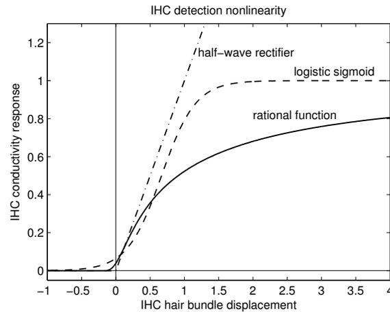
Figure 18.2: The transduction nonlinearity of the IHCs is some kind of a *sigmoid*, such as a displaced logistic function (dashed), and is sometimes modeled as simply a half-wave rectifier (dash-dot line). Other functional forms can also be used; for example, a constant segment at zero response, connected to a rational function (ratio of cubic polynomials) for the rest (solid curve), giving a cubic foot shape, a nearly linear middle region, and a slowly saturating shoulder.
