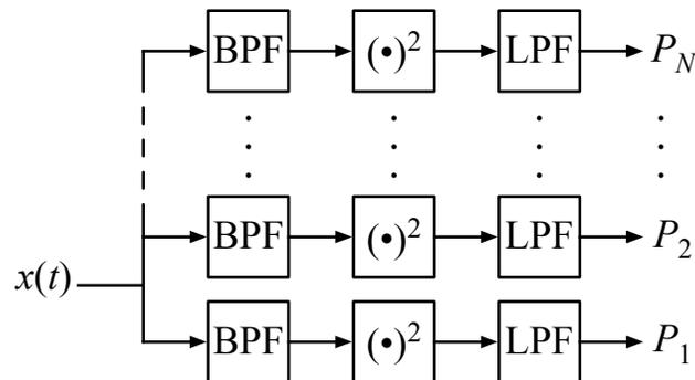
Figure 5.5: The short-time spectrum of a signal  $x(t)$  can be computed by a bank of bandpass filters (BPF), followed by squaring to detect instantaneous power, and finally lowpass filters (LPF) that establish the smoothing time scale. An  $N$ -point spectrum is made via  $N$  different BPFs with different center frequencies, and often different bandwidths, and  $N$  usually identical LPFs.
