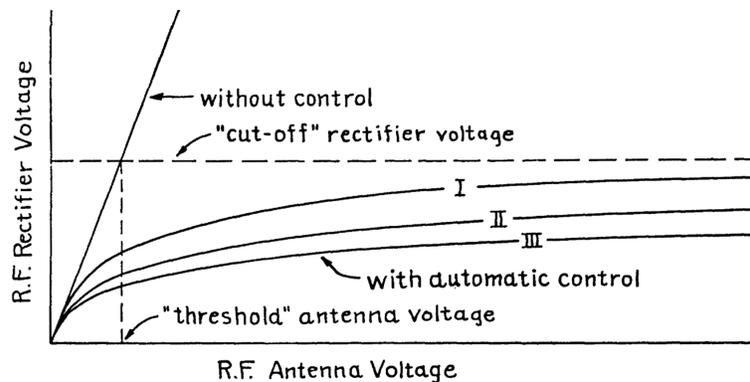
Figure 11.6: The input–output level curves of Wheeler (1928), for systems with one, two, or three cascaded variable-gain amplifiers, corresponding approximately to our model of Figure 11.5 with  $K$  values of 1 to 3. The radio-frequency output level (“R. F. Rectifier Voltage”) is almost independent of input level (“R. F. Antenna Voltage”) when the input level is well above the “threshold.” [Figure 3 (Wheeler, 1928) reproduced with permission of the IEEE.]
