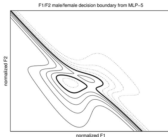
Figure 24.7: A map showing the decision boundary of a smaller MLP, classifying talker gender from  $F_1$ – $F_2$  data, along with contours of estimated class probability, in multiples of 10%. This network makes only 214 errors on the test set.
