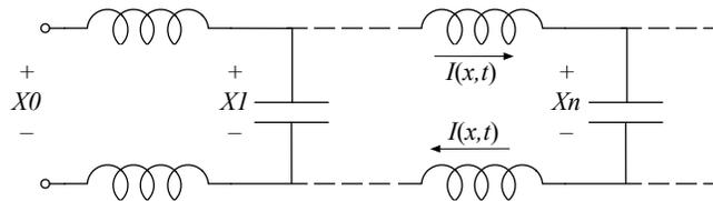
Figure 12.5: In a *balanced* or *differential* delay line, the signal of interest is the difference between the voltages on two sides, rather than with respect to a global *ground* potential. The symmetry allows such systems to be reduced to equivalent *single-ended* lines. The approximate symmetry of the hydrodynamic system of the cochlea across the cochlear partition is usually treated as good enough that the cochlea can be modeled by a single-ended transmission line circuit.
