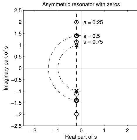
Figure 8.13: The  $s$ -plane pole-zero plot for filter D. Using mixing weight  $a = 0.5$  as shown in Figure 8.12, the zeros (shown bold) are on a circle of larger radius than that of the poles, by a factor of  $\sqrt{2}$ , and at the same  $x$  coordinate. For other mixing weights, the zeros move to other positions at the same  $x$  coordinate; examples for weights  $a = 0.25$  and  $a = 0.75$  are shown.
