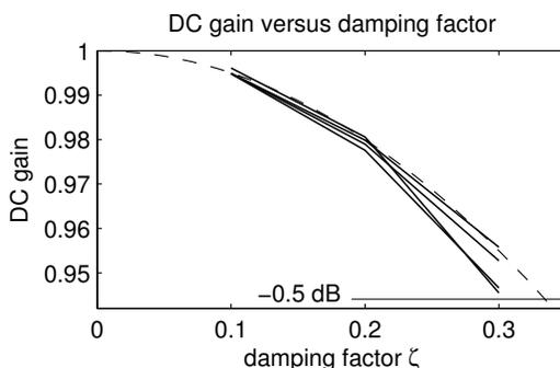
Figure 16.3: DC gains of the filter stages with pole and zero locations shown in Figure 16.2, when the gain coefficient  $g$  is fixed at the value that gives unity gain for the undamped case. The approximation  $1 - \zeta^2/2$  (dashed) is most accurate at low  $\theta_R$ . The thin line near the bottom indicates a loss of one-half dB.
